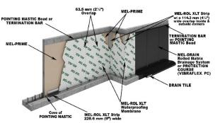
Protect the Membrane ... on all vertical and horizontal installations with the immediate application of PROTECTION COURSE (VIBRAFLEX PC) if no drainage system is used, or MEL-DRAIN. To secure PROTECTION COURSE (VIBRAFLEX PC), use POINTING MASTIC as an adhesive, and/or physically attach at the top edge using TERMINATION BAR. Backfilling should be done immediately, using care and caution to avoid damaging the waterproofing application.
