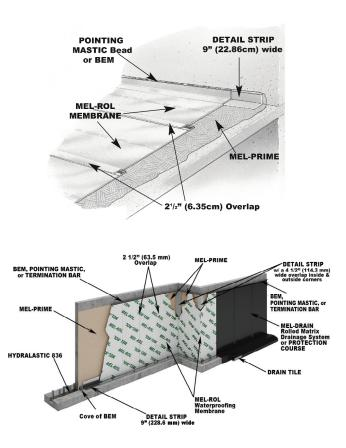
**Inspect and Repair** ... A thorough inspection should be made before covering and all necessary repairs made immediately. Tears and inadequate overlaps should be covered with MEL-ROL ... slit fish mouths and patch. Seal edges of all patches with POINTING MASTIC. Where applicable, horizontal applications can be floodtested for 24 hours. All leaks should be marked and repaired when membrane dries.
