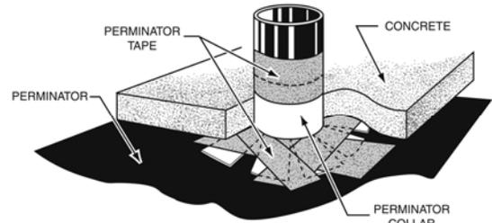
**Sealing Protrusions ...** Cut a slit around pipes, ductwork, rebar and wire penetrations to place the initial layer of the vapor barrier. To further protect the concrete slab from external moisture sources, use a piece of vapor barrier and place a collar around these as well.
