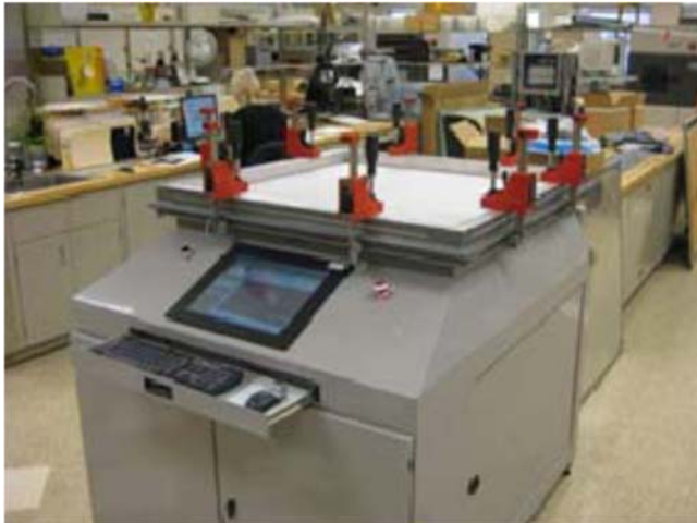
ASTM E2178 air leakage rate of building materials test being conducted
