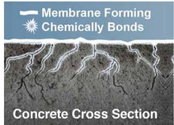
When used on fresh concrete, PENCURE OTC cures the concrete and performs similar to a post 28-day penetrating sealing compound application, offering less down time and reduced installation cost compared to what multiple coats require.
