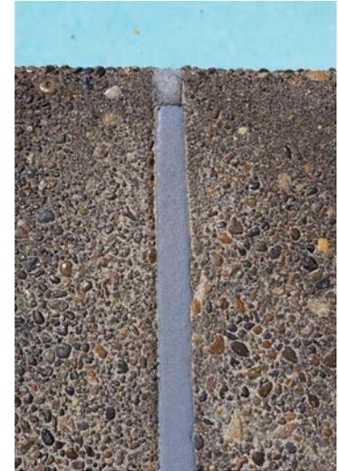
**DECK-O-SEAL two-part, polysulfide-based joint sealant is a premium-grade, pourable, self-leveling sealant. It is a non-staining sealant that cures at an ambient temperature to a firm, flexible, tear-resistant rubber. DECK-O-SEAL is highly resilient and has excellent recovery characteristics after extended periods of compression or elongation. DECK-O-SEAL is resistance to most chemicals, to all weather conditions, aging, and shrinkage.**
