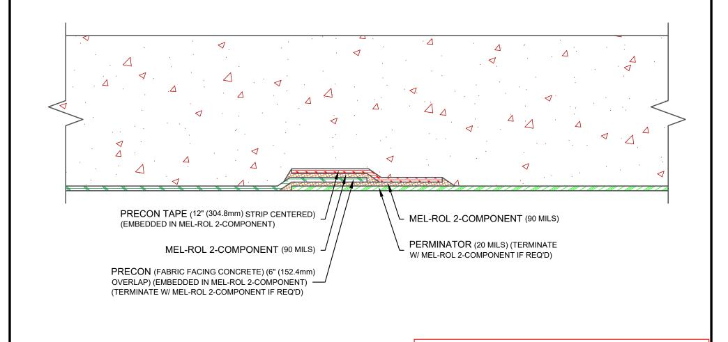
PERMINATOR (20MIL) TRANSITION TO PRECON @ UNDERSLAB
